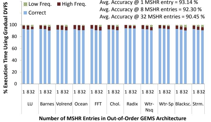
Figure 18: Gradual DVFS demonstrates high accuracy despite memory parallelism.
