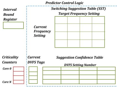
Figure 13: Our TCP hardware includes the *Criticality Counters*, *SST*, *SCT*, *Current DVFS Tags*, and *Interval Bound Register*; for a 16-core CMP with 4 DVFS levels and a threshold  $T$  of 1024, we use 71 bytes of storage overhead.
