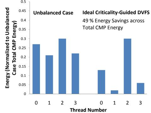
Figure 2: *Blackscholes* uses thread criticality predictors to DVFS threads, saving 49% energy without performance loss.
