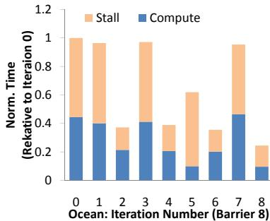
Figure 3: `Ocean`'s criticality varies with barrier iteration.
