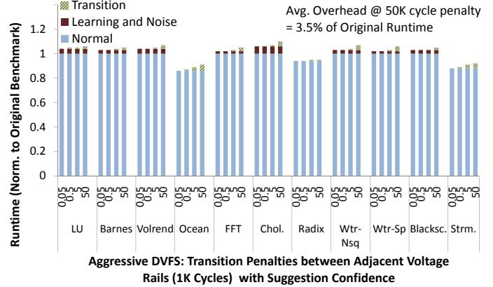
Figure 20: The *SCT* eliminates *noise* and *transition overhead*.
