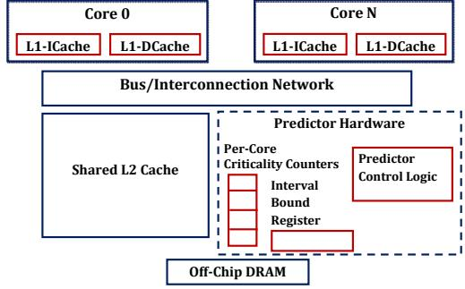
Figure 7: High-level predictor design with per-core *Criticality Counters* placed with the shared L2 cache, *Interval Bound Register*, and *Prediction Control Logic*. Hardware units are not drawn to scale.
