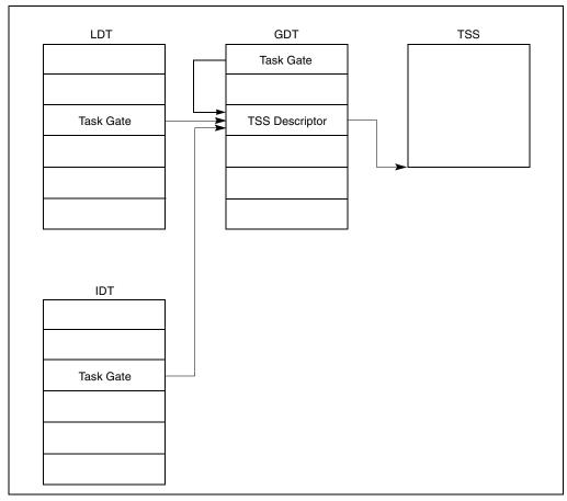
Figure 6-6. Task Gates Referencing the Same Task
