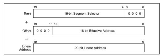
Figure 16-1. Real-Address Mode Address Translation
