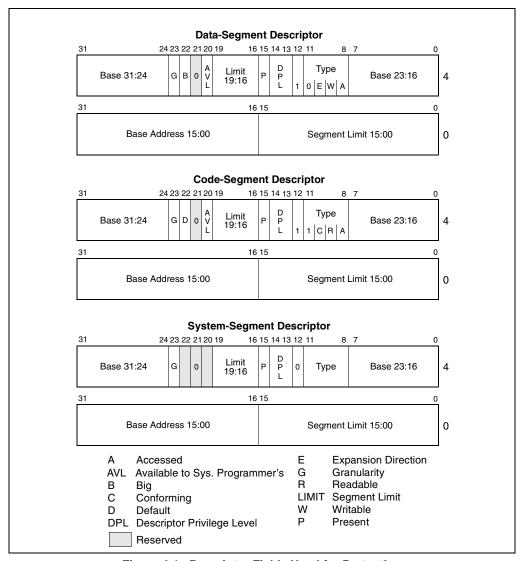
Figure 4-1. Descriptor Fields Used for Protection
