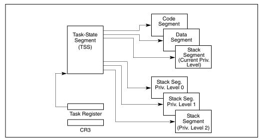
Figure 6-1. Structure of a Task
