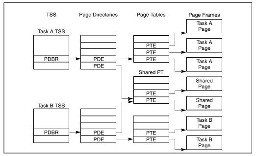
Figure 6-8. Overlapping Linear-to-Physical Mappings
