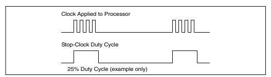
Figure 13-6. Processor Modulation Through Stop-Clock Mechanism
