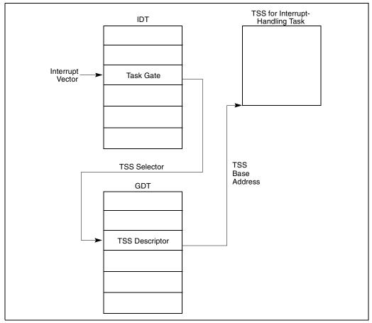
Figure 5-5. Interrupt Task Switch
