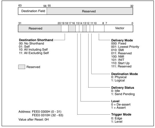
Figure 8-12. Interrupt Command Register (ICR)
