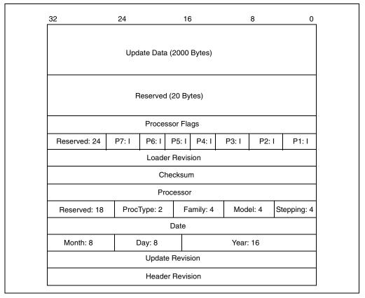
Figure 9-8. Format of the Microcode Update Data Block
