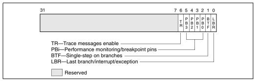
Figure 15-6. DebugCtIMSR Register (P6 Family Processors)
