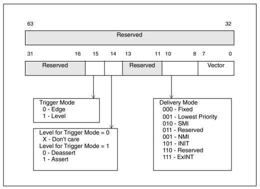
Figure 8-24. Layout of the MSI Message Data Register
