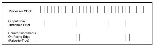
Figure 15-14. Effects of Edge Filtering
