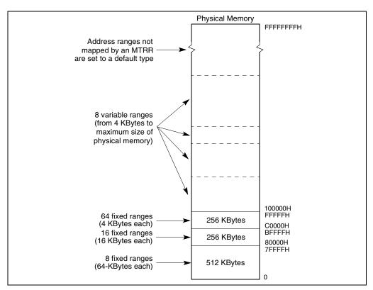
Figure 10-3. Mapping Physical Memory With MTRRs
