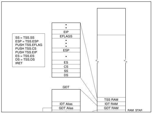
Figure 9-6. Task Switching (Lines 282-296 of List File)
