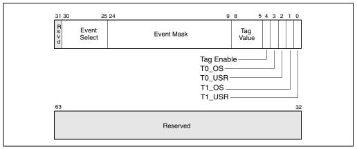
Figure 15-15. Event Selection Control Register (ESCR) for the Pentium 4 processor, Intel Xeon processor and Intel Xeon processor MP with HT Technology support
