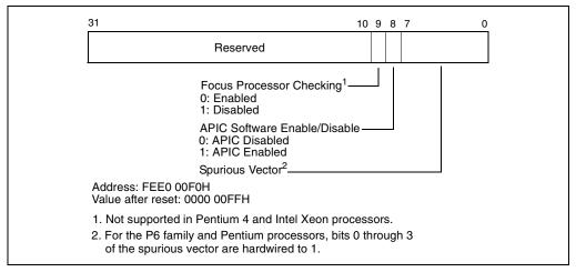
Figure 8-22. Spurious-Interrupt Vector Register (SVR)
