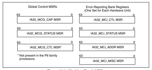
Figure 14-1. Machine-Check MSRs
