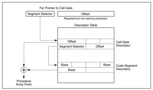
Figure 4-8. Call-Gate Mechanism
