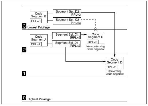
Figure 4-6. Examples of Accessing Conforming and Nonconforming Code Segments
