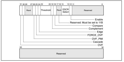
Figure 15-9. Counter Configuration Control Register (CCCR)
