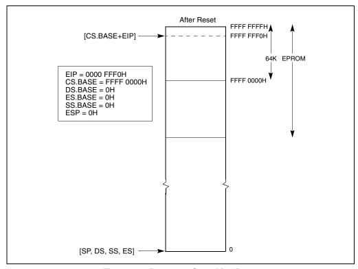
Figure 9-3. Processor State After Reset
