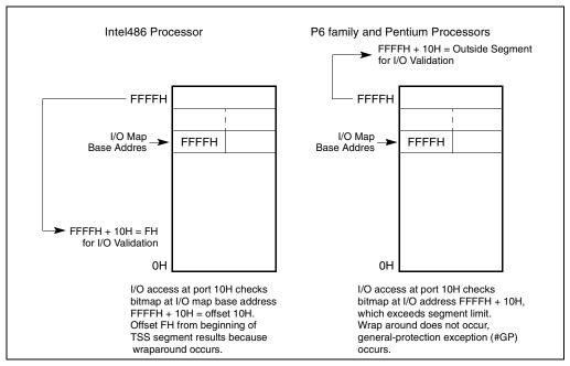
Figure 18-1. I/O Map Base Address Differences
