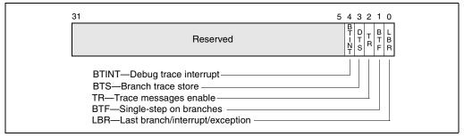
Figure 15-2. IA32\_DEBUGCTL MSR (Pentium 4 and Intel Xeon Processors)
