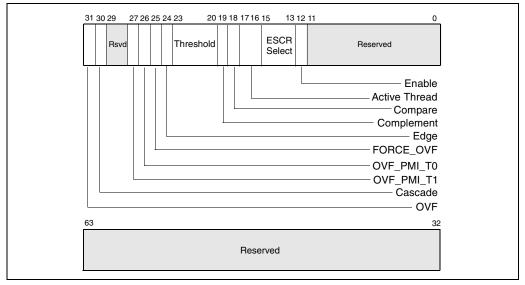
Figure 15-16. Counter Configuration Control Register (CCCR)
