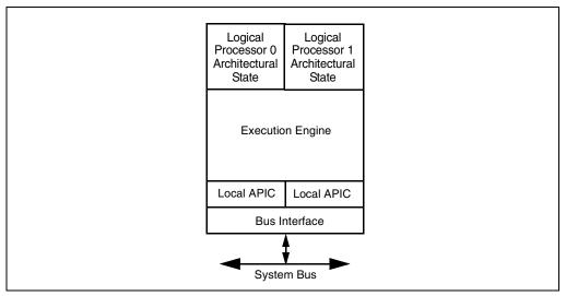
Figure 7-3. IA-32 Processor with Intel Hyper-Threading Technology using
