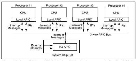
Figure 8-3. Local APICs and I/O APIC When P6 Family Processors Are Used in Multiple-Processor Systems
