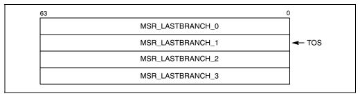
Figure 15-3. LBR MSR Stack Structure
