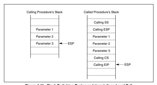
Figure 4-11. Stack Switching During an Interprivilege-Level Call
