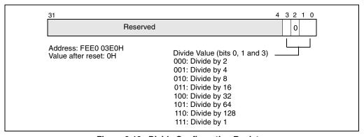
Figure 8-10. Divide Configuration Register
