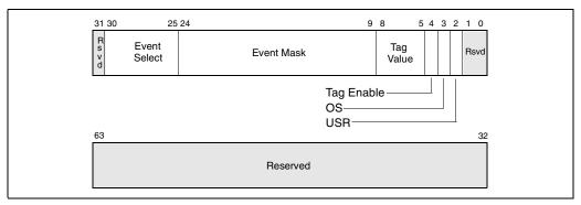
Figure 15-7. Event Selection Control Register (ESCR) for Pentium 4 and Intel Xeon processors without HT Technology support
