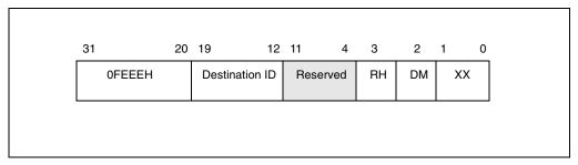
Figure 8-23. Layout of the MSI Message Address Register
