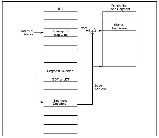
Figure 5-3. Interrupt Procedure Call
