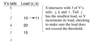
Figure 7. Balance condition example.
