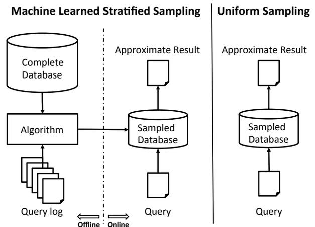
**Figure 1: Standard architecture for database sampling. Our algorithm determines sampling probabilities for individual records based solely on a historical query log.**
