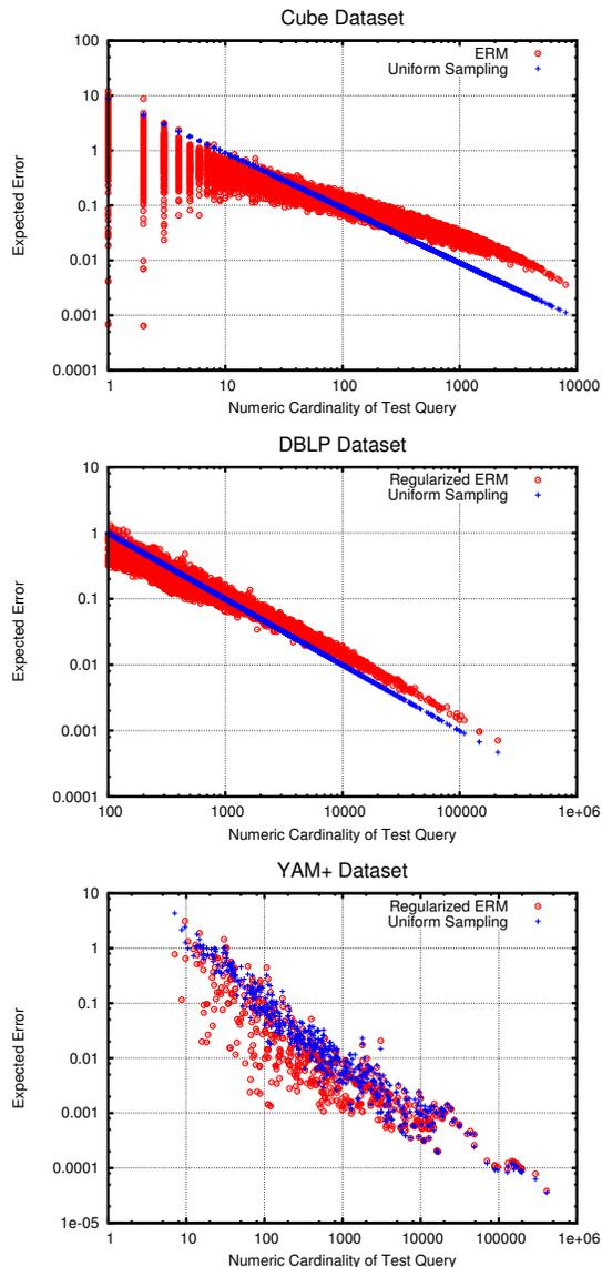
**Figure 4:** These three plots show the expected error of each test query. Clearly, for all three datasets, error is a generally decreasing function of the numeric cardinality of the queries. The advantage of ERM over uniform random sampling lies primarily at the more difficult low cardinality end of the spectrum.
