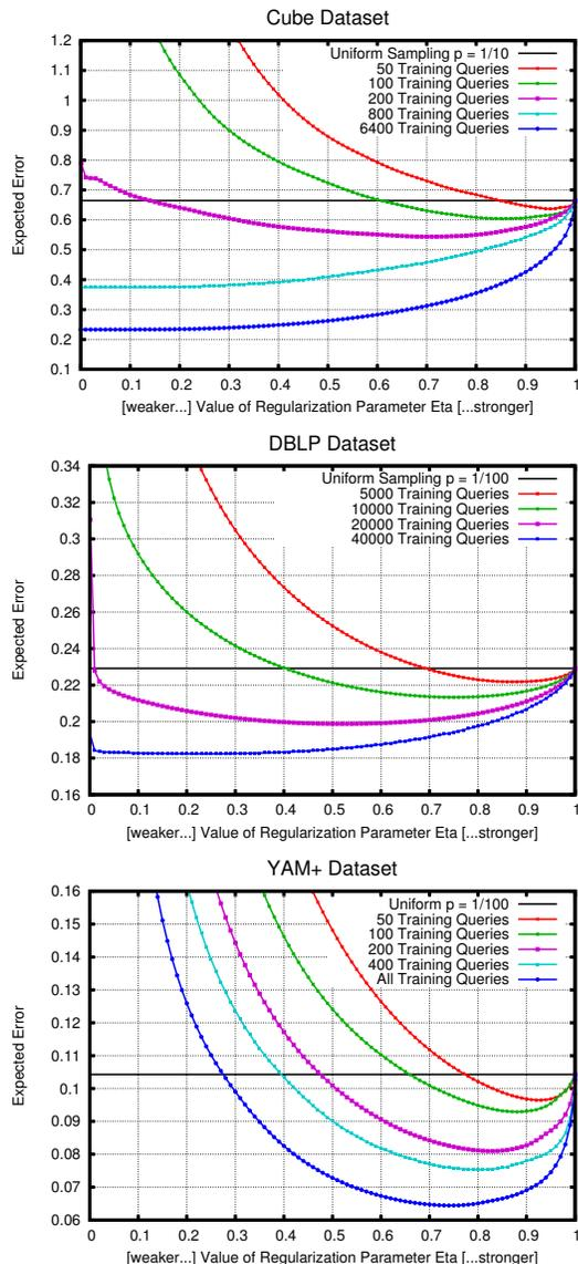
**Figure 3:** The three plots correspond to the three datasets. The  $y$ -axis is the average expected normalized squared error on the testing queries (lower values are better). The different curves in each plot correspond to different sizes of training sets (see the legend). The black horizontal line corresponds to uniform sampling using a similar sampling rate. The value of  $\eta$  (strength of regularization) varies along the  $x$ -axis.
