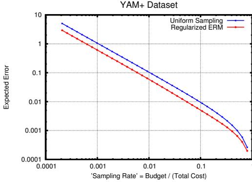
**Figure 5: ERM with mixture regularization versus uniform random sampling at various effective sampling rates ( $B/\sum c_i$ ).** The gains might appear unimpressive in the log-log scale plot but are, in fact, 40%-50% throughout which is significant.
