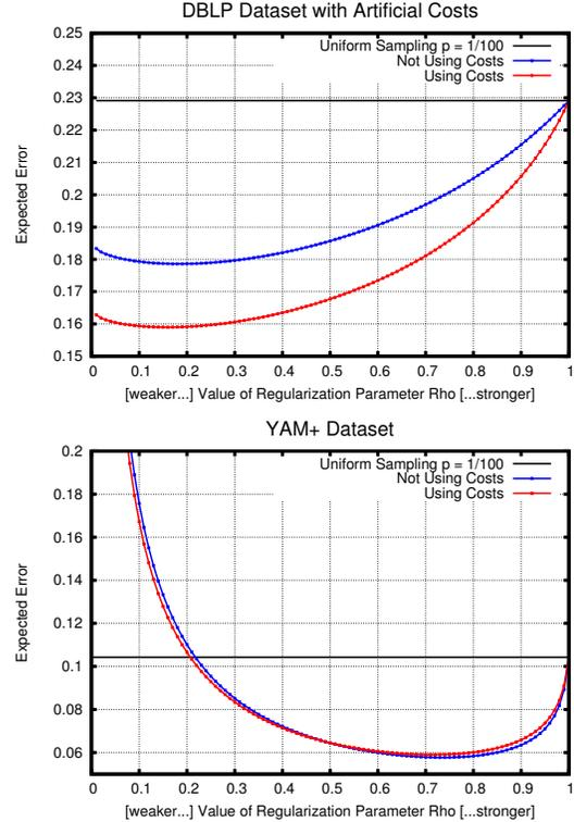
**Figure 6: These plots show the effect of taking the costs  $c_i$  into account while computing the values  $z_i$ .** For YAM+, record costs correspond to the size of the record on disk. For the DBLP dataset randomly generated artificial record costs were used.
