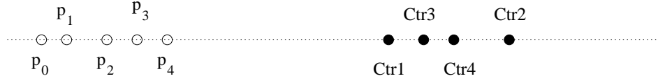
Figure 3.4: A point may be moved in each rounding, but all the displacements are in the same direction.
