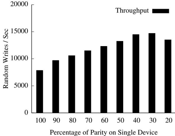
**Figure 12.** Diff-RAID throughput under various parity assignments.
