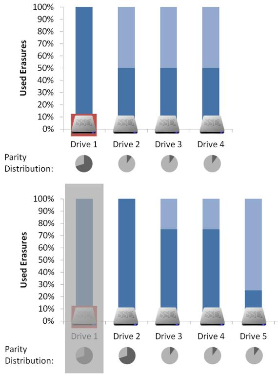
**Figure 3.** Parity-Shifting Drive Replacement for a 4-device array with parity assignment (70, 10, 10, 10): age distribution of devices when Drive 1 is replaced (Top), and when Drive 2 is replaced (Bottom). Drive 2 receives 70% of the parity after Drive 1 is replaced.
