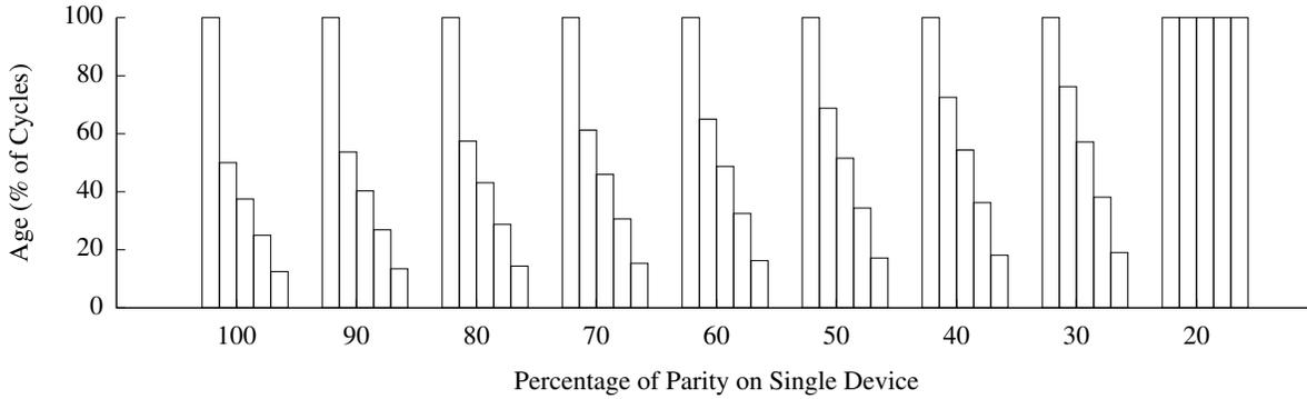
**Figure 5.** Convergent distribution of ages at replacement time for different parity assignments; on the x-axis is the percentage of parity on a single device, with the rest spread evenly across the other devices (e.g.,  $x = 60$  represents  $(60, 10, 10, 10, 10)$ ).
