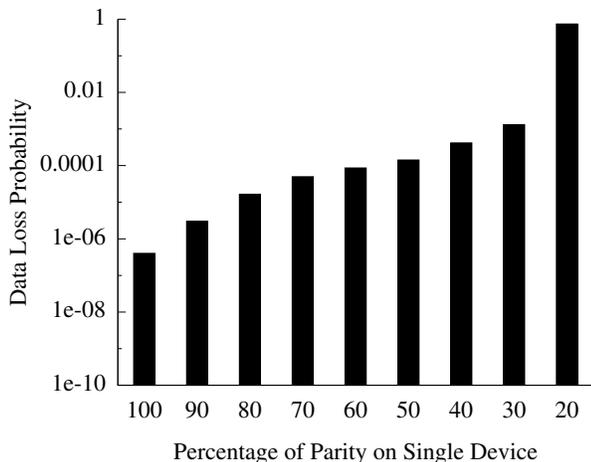
**Figure 7.** Diff-RAID provides tunable reliability. X-axis shows % of parity on first device, with remaining parity divided evenly across other devices. Left-most bar corresponds to (100, 0, 0, 0, 0) and right-most to (20, 20, 20, 20, 20).
