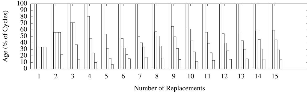
**Figure 4.** Distribution of device ages at replacement time for  $(80, 5, 5, 5, 5)$  parity assignment: on each replacement, a new device is added to the end of the array and the second device moves into first position.
