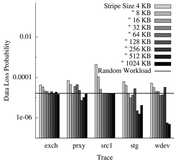
**Figure 11.** Diff-RAID reliability with different traces and stripe sizes shows that there’s no universally good stripe size, but Diff-RAID works well with different workloads if the stripe size is selected carefully.
