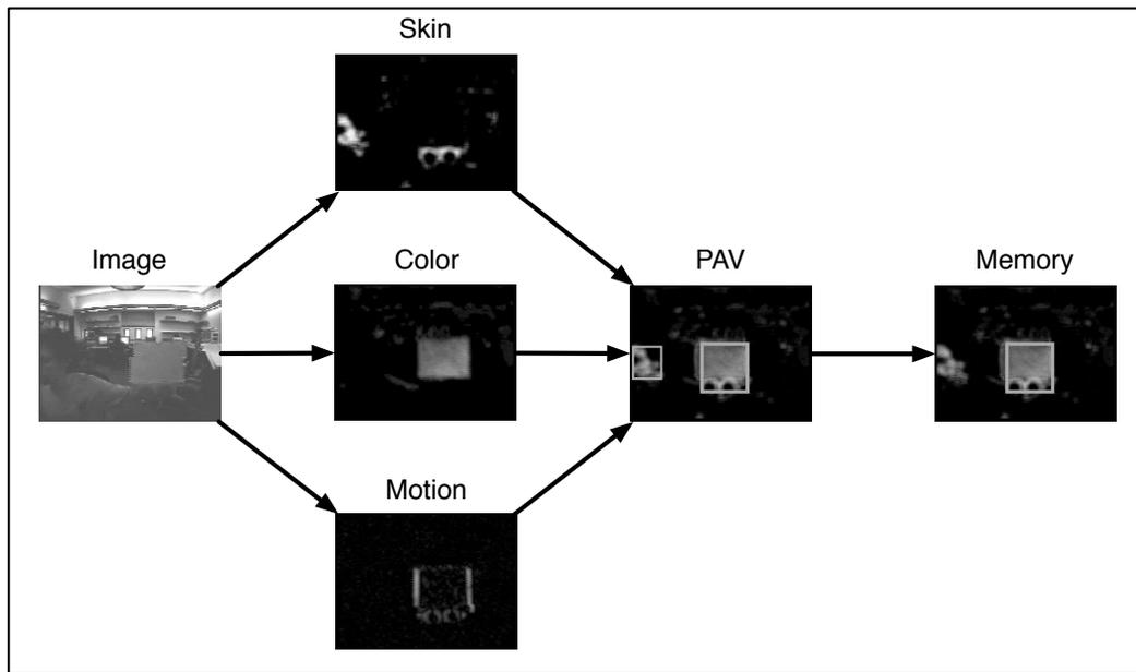
**Figure 2. The Visual Processing Pipeline: the image is passed to the Skin, Color, and Motion modules, each of which produces a saliency map; the PAV module performs a weighted summation of their output and boxes interesting objects; the *memory* module performs habituation and chooses the most salient object (the images shown above represent typical output from each module)**
