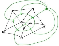
There are many powerful characterizations of planar graphs. I'll now introduce my favorite by introducing a way of drawing a planar graph, which turns out to be a way of drawing any planar graph.
