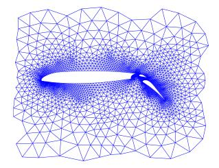
We will now draw it using coordinates from the eigenvectors. I will plot vertex u at point  $(\psi_2(u), \psi_3(u))$  I will draw the edges as straight lines between the vertices they connect.
