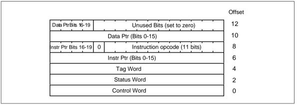
Figure 14.11 FPU Environment Record (16 Bit Real Mode)
