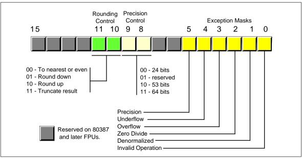
Figure 14.6 80x87 Control Register
