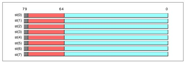
Figure 14.5 80x87 Floating Point Register Stack
