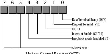
Modem Control Register (MCR)
