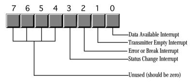
Serial Port Interrupt Enable Register (IER)
