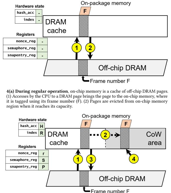
Figure 4: Layout of on-chip memory.
