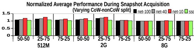
**Figure 12: Performance impact of snapshot acquisition for different CoW-Cache partitions.** Y-axis shows average performance impact of all benchmarks to take a snapshot, varying CoW-nonCoW partition for different cache sizes. X-axis shows different total sizes of die-stacked memory and various ways in which to partition die-stacked memory for CoW (50%, 25% and 75% for CoW).
