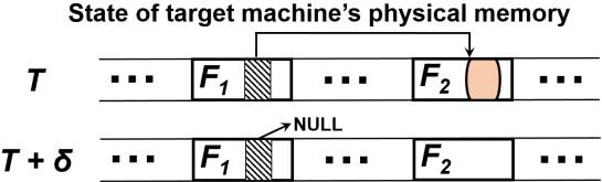
**Figure 3: Example showing need for snapshot consistency.** Depicted above is the memory state of a target machine at two points in time,  $T$  and  $T+\delta$ . At  $T$ , a pointer in  $F_1$  points to an object in  $F_2$ . At  $T+\delta$ , the object has been freed and the pointer set to `NULL`. Without consistency, the snapshot could contain a copy of  $F_1$  at time  $T$  and  $F_2$  at time  $T+\delta$  (or vice-versa), causing problems for forensic analysis.
