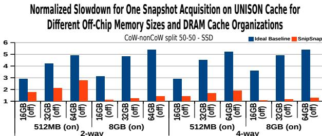
**Figure 13: Performance as size and set-associativity of UNISON cache changes.** Lower UNISON cache size and set-associativity increases the chances that a set in the CoW region fills up and pauses execution of applications on the target. Results are shown using SSDs, varying off-chip DRAM capacity from 16GB to 64GB, UNISON cache size from 512MB to 8GB, and set-associativity from 2 to 4 way.
