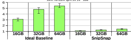
**Figure 9: Average performance with varying off-chip DRAM size.** Bigger off-chip DRAM takes longer to snapshot, so SnipSnap becomes even more advantageous over current idealized approaches. These results assume UNISON cache with 8GB, split 50:50 in CoW:non-CoW mode during snapshot acquisition and SSDs, taking just one snapshot.
