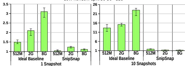
**Figure 8: Performance impact of snapshot acquisition from simulator studies with UNISON cache [52].** SnipSnap outperforms idealized versions of current snapshotting approaches by as much as 22× (graphs show benchmark averages, maxima, and minima).
