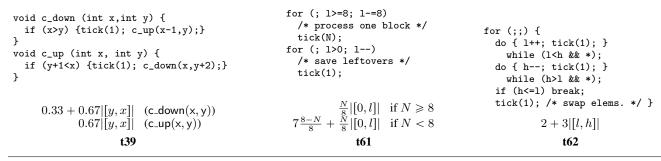
Figure 3. Example t39 shows two mutually-recursive functions with the computed tick bounds. Example t61 and t62 demonstrate the unique compositionality of our system. In t61,  $N \ge 0$  is a fixed but arbitrary constant.
