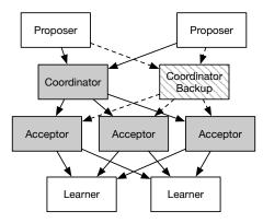
Figure 3: A switch-based deployment of CAANS. Switch hardware is shaded grey, and commodity servers are colored white. The arrows represent communication. The coordinator backup may be deployed on either switch hardware of a commodity server. The dashed-arrows represent backup communication.
