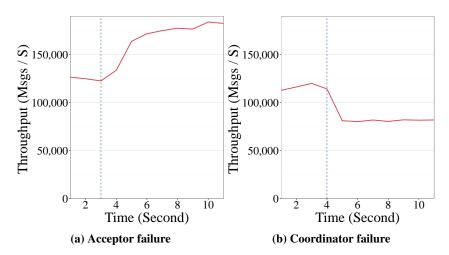
Figure 8: The performance of CAANS when (a) an acceptor fails, and (b) when the hardware coordinator fails and is replaced by a software coordinator.
