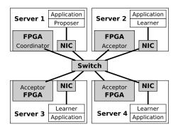
Figure 6: An implementation of CAANS using FPGAs.
