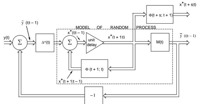
Fig. 3 Matrix block diagram of optimal filter
