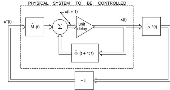
Fig. 4 Matrix block diagram of optimal controller
